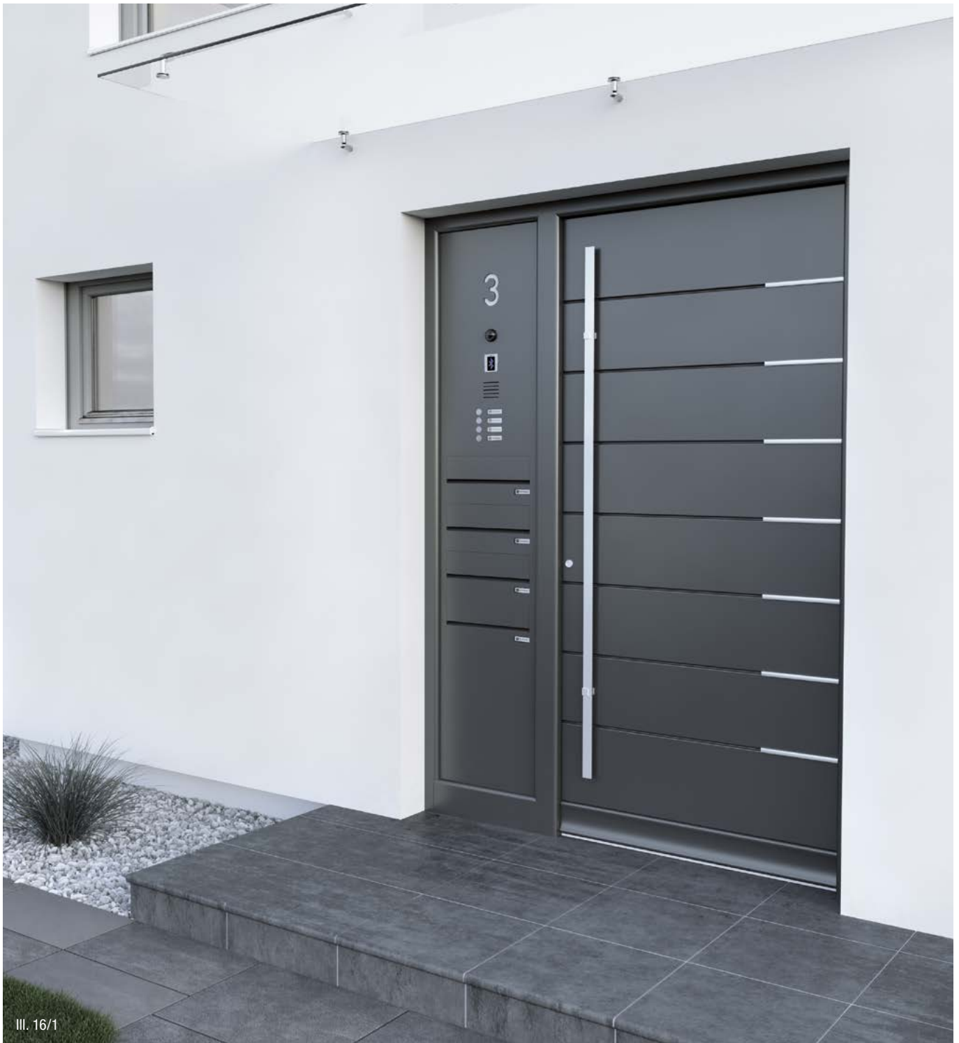
First Class fully insulated door side system model 02-941 ISO aluminium front plate and mail slot flap I/D compartment with intercom grid 21-174 doorbell button 21-216FW name plate 21-134 module preparation for modules to be supplied by the customer (fingerprint, camera) House number engraving flush with milky acrylic glass and illuminated with LED
