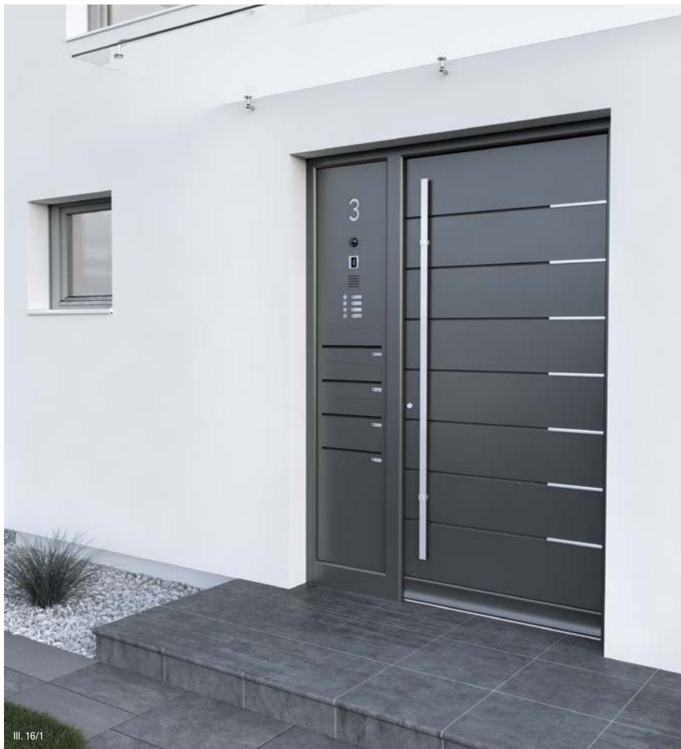
III. 16/1 First Class fully insulated door side system model 02-941 ISO aluminium front plate and mail slot flap I/D compartment with intercom grid 21-174 doorbell button 21-216FW name plate 21-134 module preparation for modules to be supplied by the customer (fingerprint, camera) House number engraving flush with milky acrylic glass and illuminated with LED
