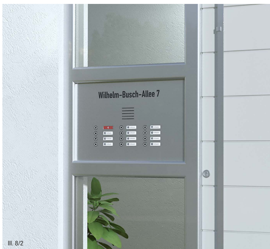
Doorbell panel with aluminium front plate thermally isolated intercom grid 21-174 doorbell button 21-216FW with name plate 21-134 street/house number engraving and illuminated
